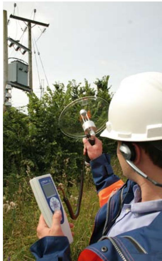
Listen for PD activity in overhead assets with the UltraDish™ add-on.
