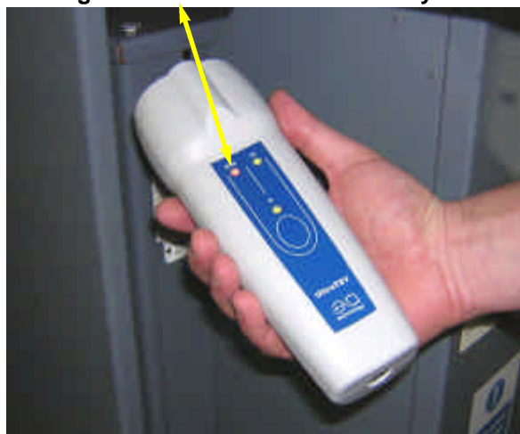
Red light indicates ultrasonic activity
